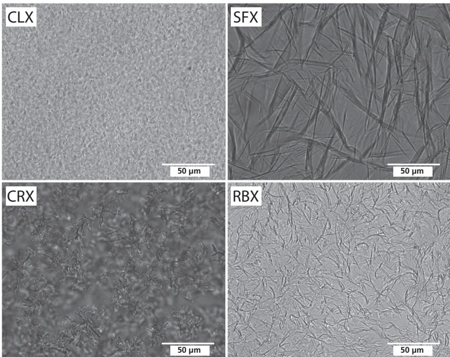
**Figure 10.4** Brightfield light micrographs of wax–oil gels consisting of 10% wax (w/w) in canola oil at a temperature of 25 °C. The different waxes are labeled as follows: candelilla wax (CLX), carnauba wax (CRX), sunflower wax (SFX), and rice bran wax (RBX).
