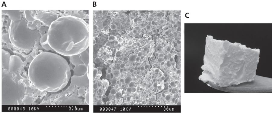
**Figure 10.1** (A, B) Cryo-scanning electron micrographs of a structured oil-in-water emulsion, similar to the commercial product Coasun™. (C) Structured emulsion Coasun™, which can possess a shortening-like texture through the use of a surfactant and careful control of pH. Coasun™ can successfully be used for a variety of baking applications by replacing traditional fats high in saturated and TFAs.
