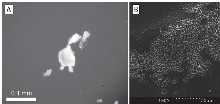
**Figure 10.9** (A) Polarized light micrograph of 10 cP ethylcellulose powder in water. (B) A cryo-scanning electron micrograph of a canola oil organogel using 45 cP ethylcellulose, treated with 3.4 mL of isobutanol to remove surface oil.
