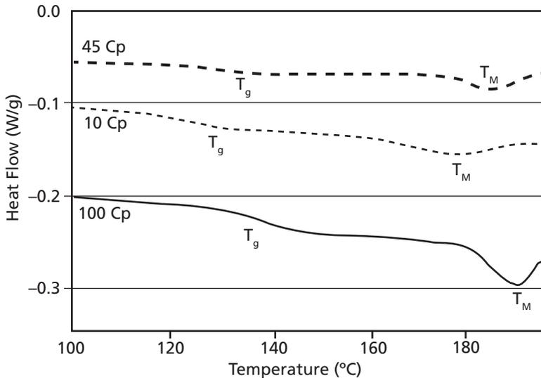
**Figure 10.7** Sample differential scanning calorimetry thermogram showing the glass transition and melting for 10, 45, and 100 cP ethylcellulose powder.
