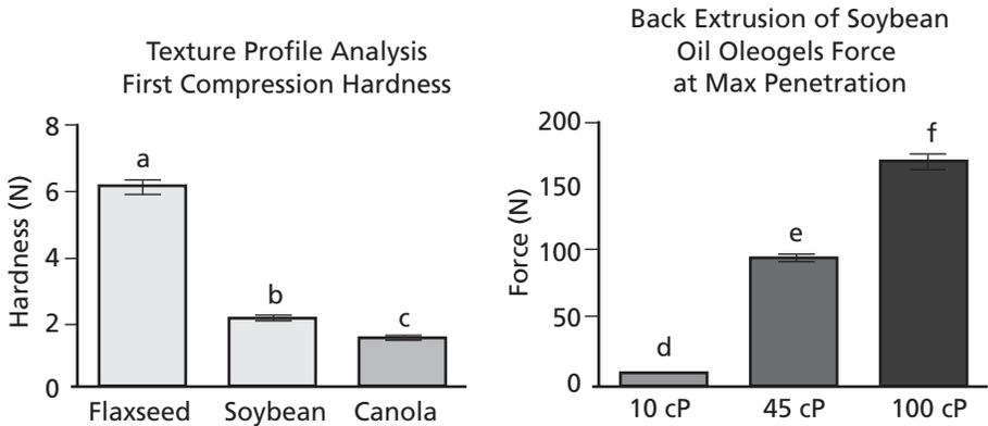
**Figure 10.8** Texture profile analysis and back extrusion results for testing the mechanical properties of oleogels made with 10% ethylcellulose (w/w) in vegetable oil. The texture profile analysis results show the effect of oil type on hardness, while the back extrusion results illustrate the differences in hardness due to ethylcellulose molecular weight.
