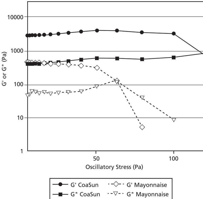
**Figure 10.3** Storage modulus ( $G'$ ) and loss modulus ( $G''$ ) for the structured emulsion CoaSun™ and a typical oil-in-water emulsion, mayonnaise, over a range of oscillatory stresses.
