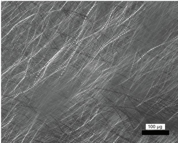
**Figure 10.5** A polarized light micrograph showing the fibrillar crystals of 12-hydroxystearic acid in canola oil at a concentration of 2.5% (w/w).
