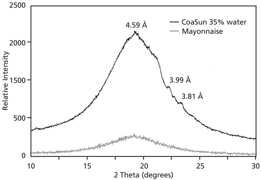
**Figure 10.2** Small and wide angle X-ray diffraction spectra for CoaSUN™ and mayonnaise.
